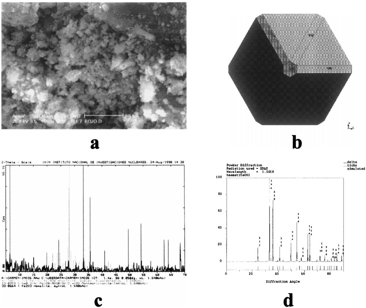
Figure 4 Results obtained for the red pigment which is composed by hematite ( $\text{Fe}_2\text{O}_3$ ). a) SEM secondary electron image showing the crystals. b) The expected habit for the hematite crystals. c) Experimental X-ray diffraction pattern of the red pigment. d) calculated X-ray diffraction pattern for hematite showing agreement with the one referred in c).
